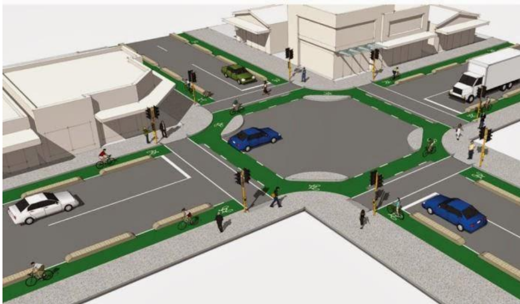
Figure 29: Urban intersection with cycle lanes and sidewalks
