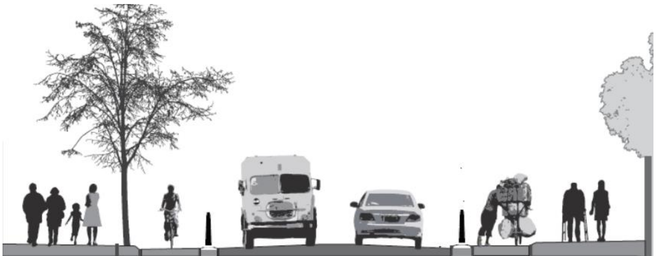
Figure 23: Typical cross-section of urban collector roads
