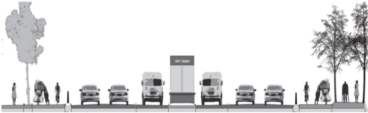
Figure 22: Typical cross-section of urban arterials
